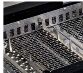
Under board support pins. Standard accessory. It consists of two rail and four pins.
